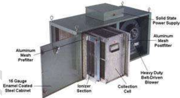
Gambar 23. Electrostatic Precipitator (CEPIC, 1999)
